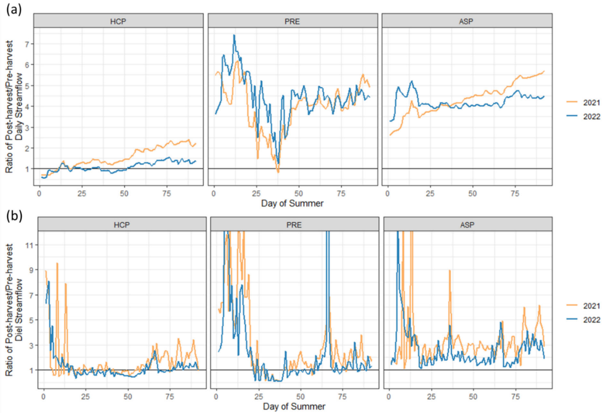
Figure A.3. Ratio of post- to pre-harvest streamflow in each treated stream each day through the summer. (a) Ratio of post- to pre-harvest total daily streamflow. (b) Ratio of post- to pre-harvest diel streamflow.
