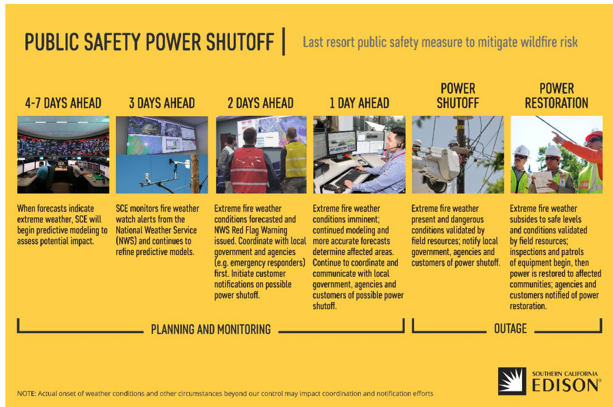
Figure 86: SCE Public Safety Power Shutoff Process
