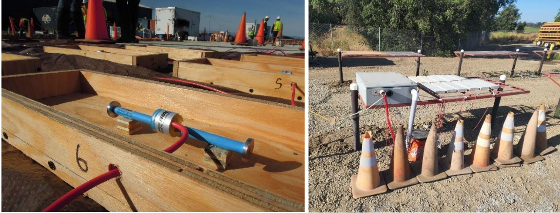
Figure 26. Unrestrained shrinkage prisms
