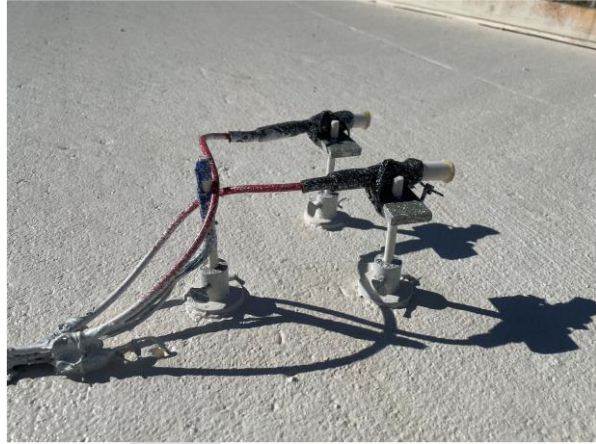
Figure 27. Test section instrumentation; left: thermocouple rod and pair of VWSFs; right: thermocouple rod and two RH sensors
