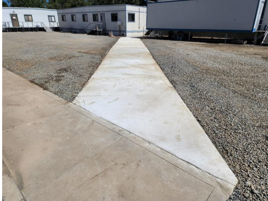
Figure 22. Test sections (from picture bottom to top: PLC, CNC, and OPC)
