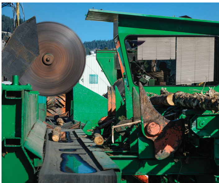
Heartwood Biomass processes firewood on a bucking saw with a merchandizing line. Photo courtesy of Heartwood Biomass
