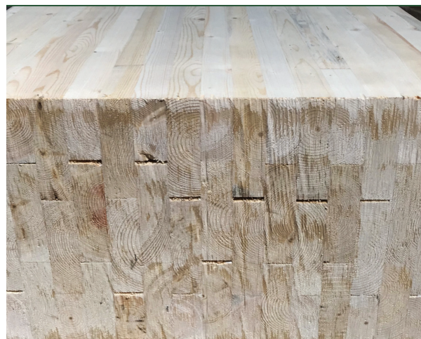
Figure 3. Glulam cross-section. Photo courtesy of ThinkWood ( https://www.thinkwood.com/mass-timber/glulam )
