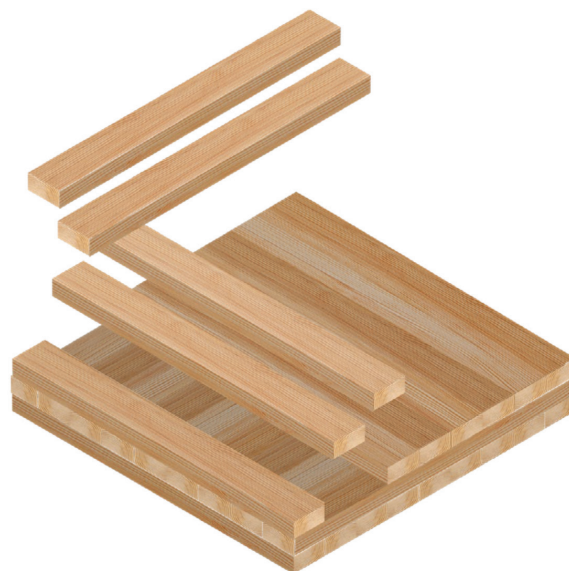
Figure 2. Cross-laminated timber layers. Image from the 2021 Mass Timber Design Manual, courtesy of WoodWorks and ThinkWood ( info.thinkwood.com/masstimberdesignmanual )
