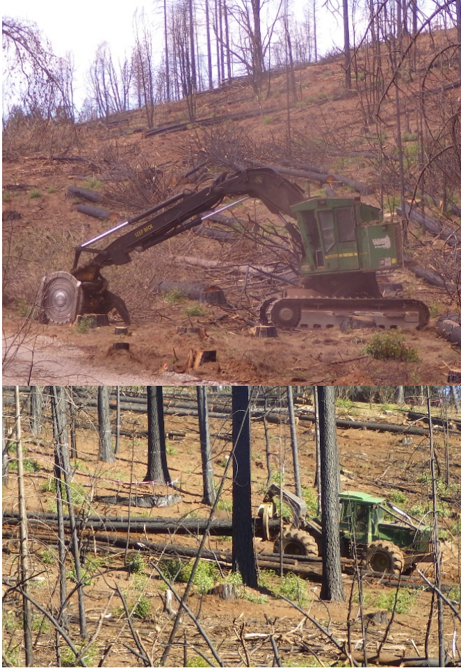
Figure 3.1: A feller buncher (top) and a wheeled log skidder retrieving a bundle of trees (Bottom).
