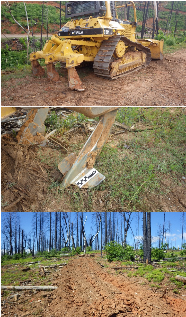
Figure 3.5: Bulldozer equipped with shanks for subsoiling (Top), close up of "winged" shanks from the opposite perspective (Middle), and subsoiled skid trail (Bottom).
