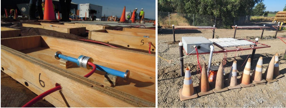
Figure 26. Unrestrained shrinkage prisms
