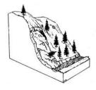
**DEBRIS FLOW:** A Soil Flow where the majority of the materials are coarse-grained (fine sand to boulder size particles) and non-cohesive. Debris flows are most often triggered by intense rainfall following a period of less intense precipitation, or by rapid snow melt.
