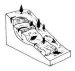
**EARTH FLOW:** A specific type of Soil Flow landslide where the majority of the soil materials are fine-grained (silt and clay) and cohesive. The material strength is low through much of the slide mass, and movement occurs on many discontinuous shear surfaces throughout the landslide mass.
