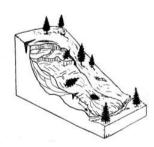
**DEBRIS SLIDE**: A slide of coarse-grained soil, most common in unconsolidated sandy or gravelly units, but also are common in residual soils that form from in-place weathering of relatively hard rock. Owing to the granular constituents, overall strength of the debris slide mass generally is higher than that of earth flows, but there may be a very low strength zone at the base of the soil or within weathered bedrock.
