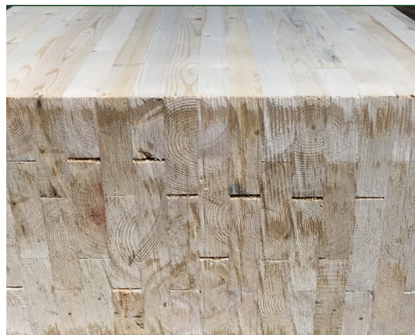
Figure 3. Glulam cross-section. Photo courtesy of ThinkWood ( https://www.thinkwood.com/mass-timber/glulam )
