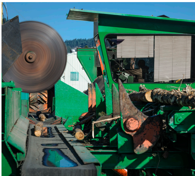
Heartwood Biomass processes firewood on a bucking saw with a merchandizing line. Photo courtesy of Heartwood Biomass
