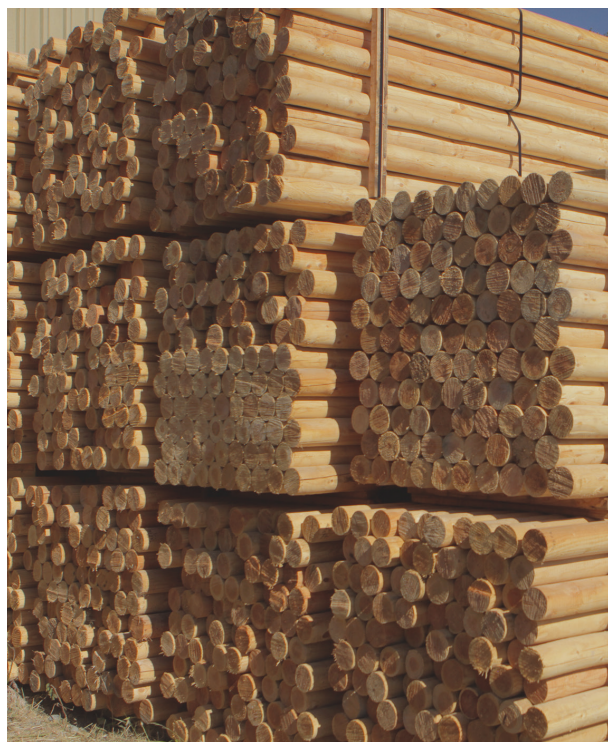
Stacked poles after debarking and processing
