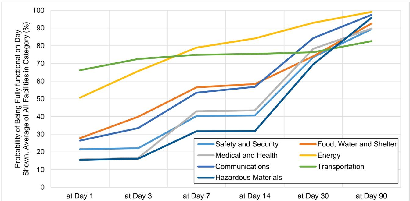
**Figure 9-21. Critical Facility Functionality, Rodgers Creek – Healdsburg Fault Scenario**
