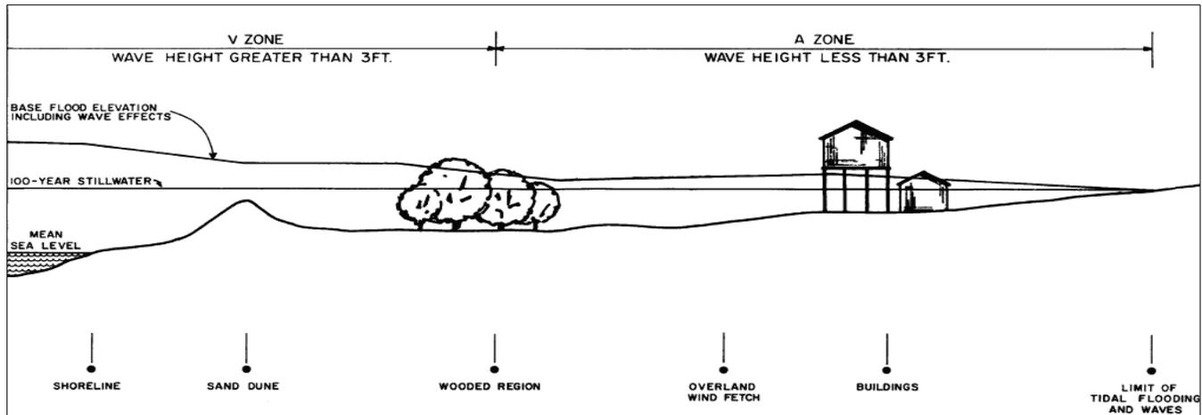
**Figure 10-1. Typical Transect Schematic**
