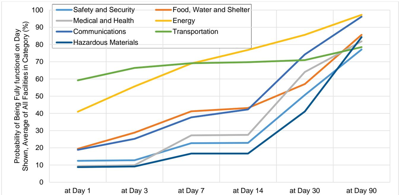
**Figure 9-19.** Critical Facility Functionality, Hayward Fault Scenario
