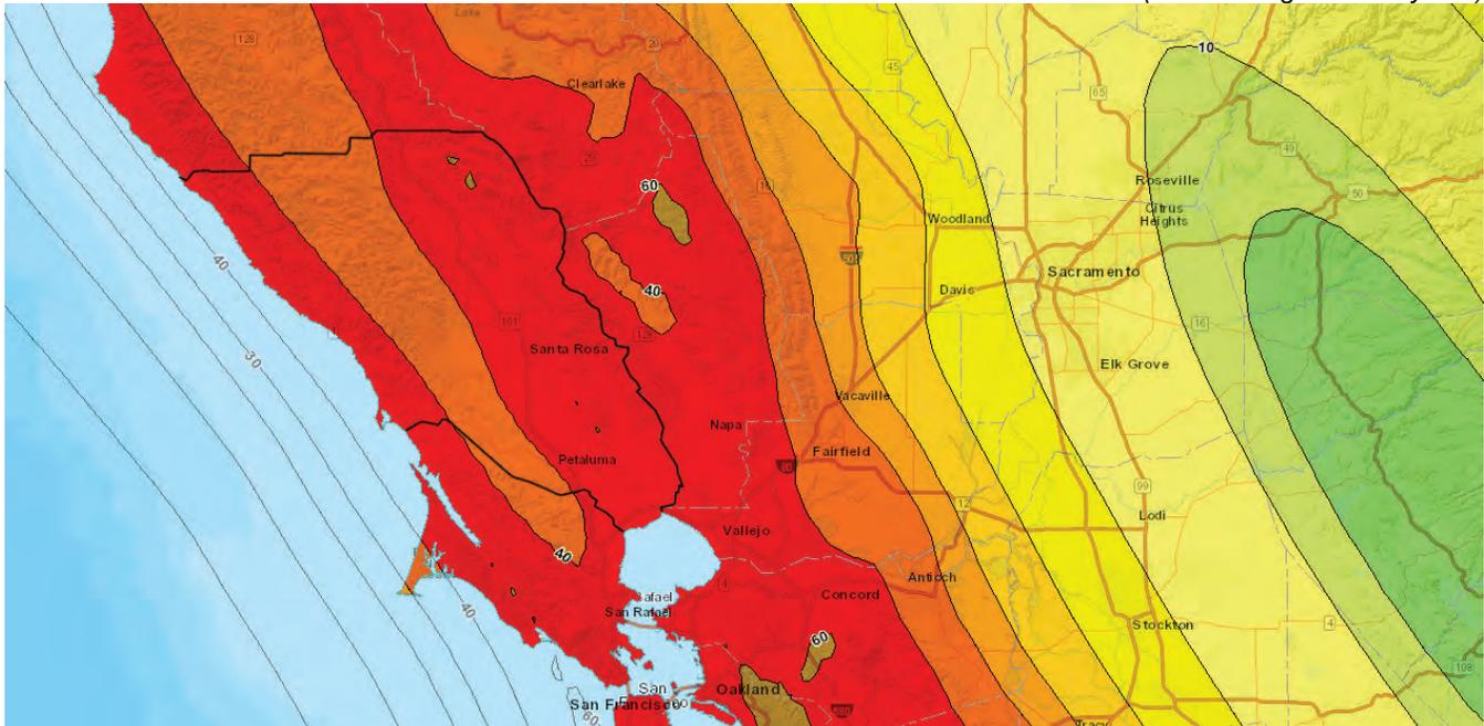
**Figure 9-5. Peak Horizontal Acceleration (%g) with 10% Probability of Exceedance in 50 Years**
