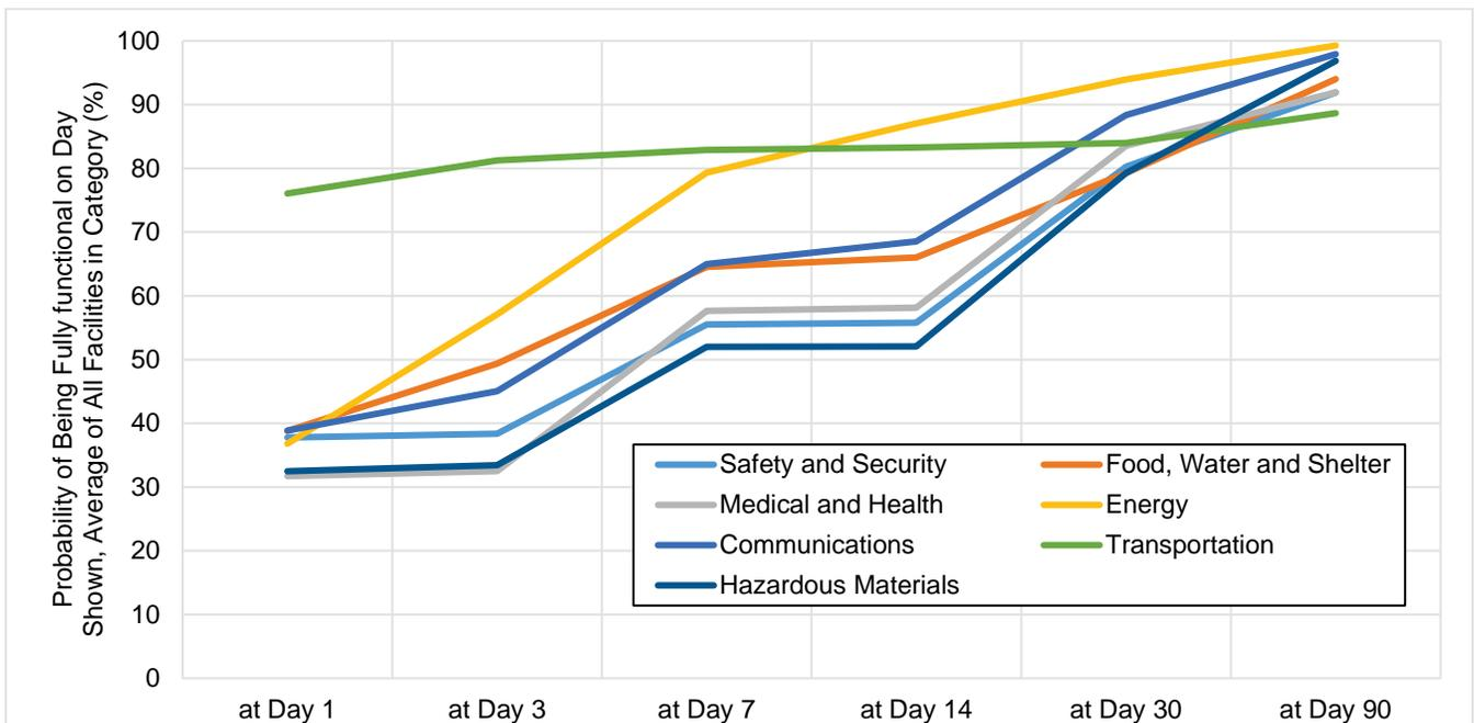
**Figure 9-20.** Critical Facility Functionality, Maacama Fault Scenario
