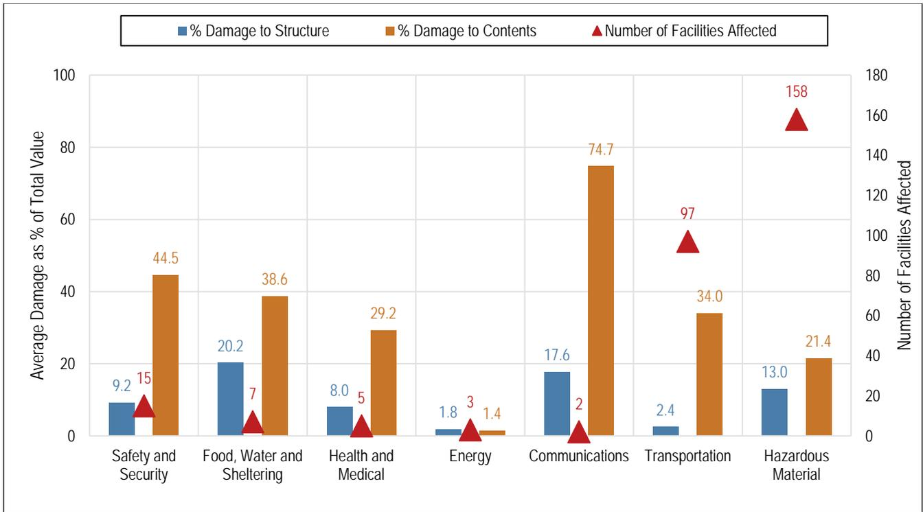
**Figure 10-7. Estimated Damage to Critical Facilities from 1% Annual Chance Flood**
