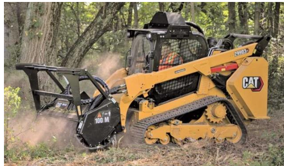
Figure 9: Example of Mechanized Equipment - 299 CAT
