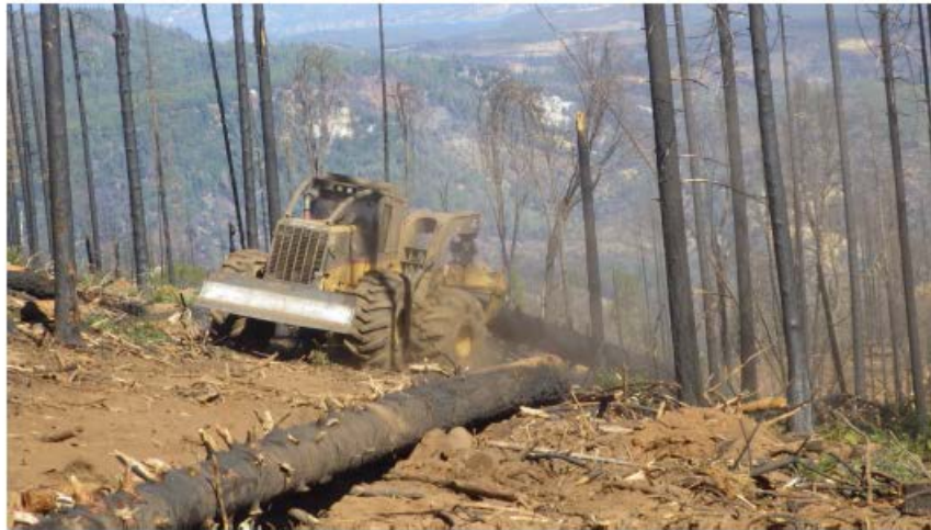
Rubber-tired skidder operating after the 2015 Valley Fire on the Boggs Mountain Demonstration State Forest in Lake County, California.
