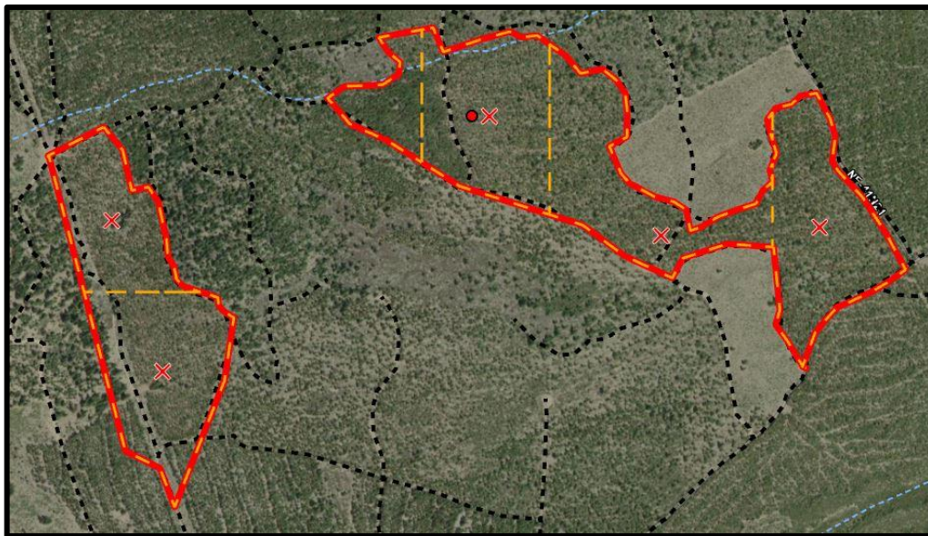
Figure 10: An FFP example of sampling on a Notice over 80 acres in size, with the GIS mapped boundaries shown (red solid line), plot centers shown by red x's, and the centroid shown by a red dot. Orange dashed lines indicate “block” boundaries.
