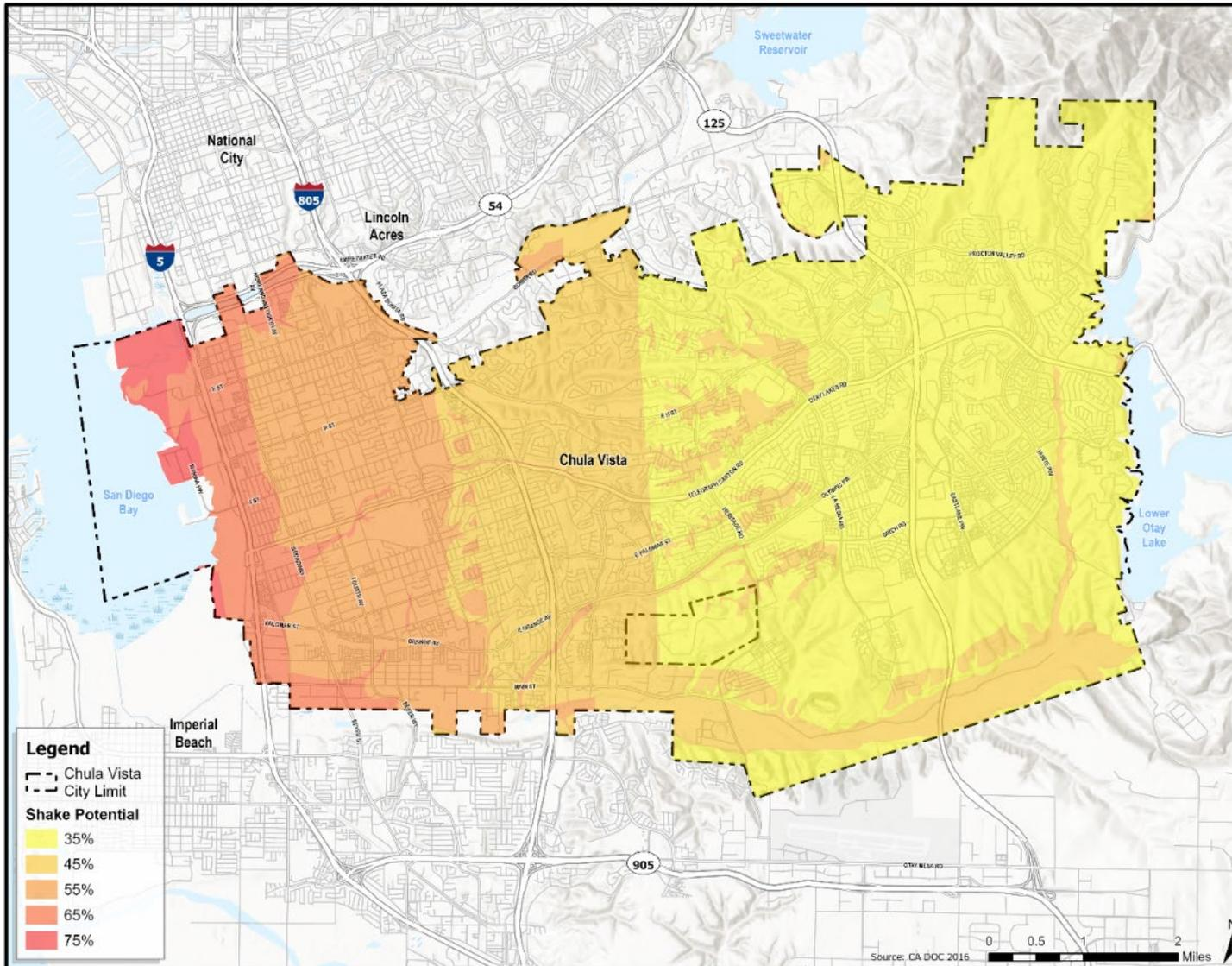
Figure 5: Liquefaction Zones
