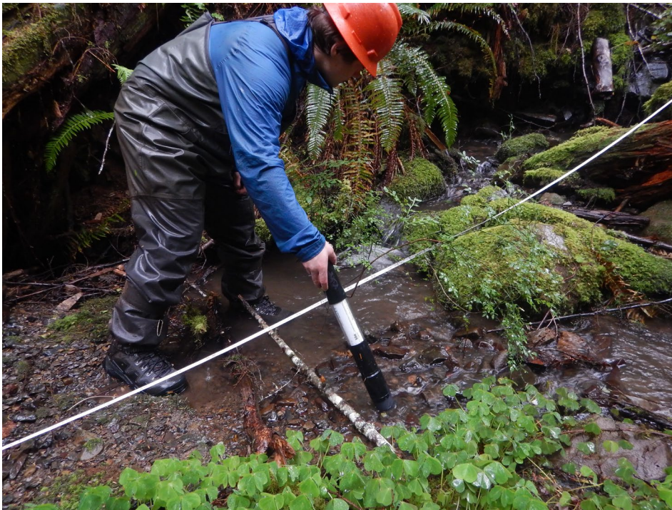
Measuring algal concentrations with a BentoTorch at a study site in a lower Klamath River tributary for the of Class II riparian prescription effectiveness study. Photo by Jonah Nicholas.
