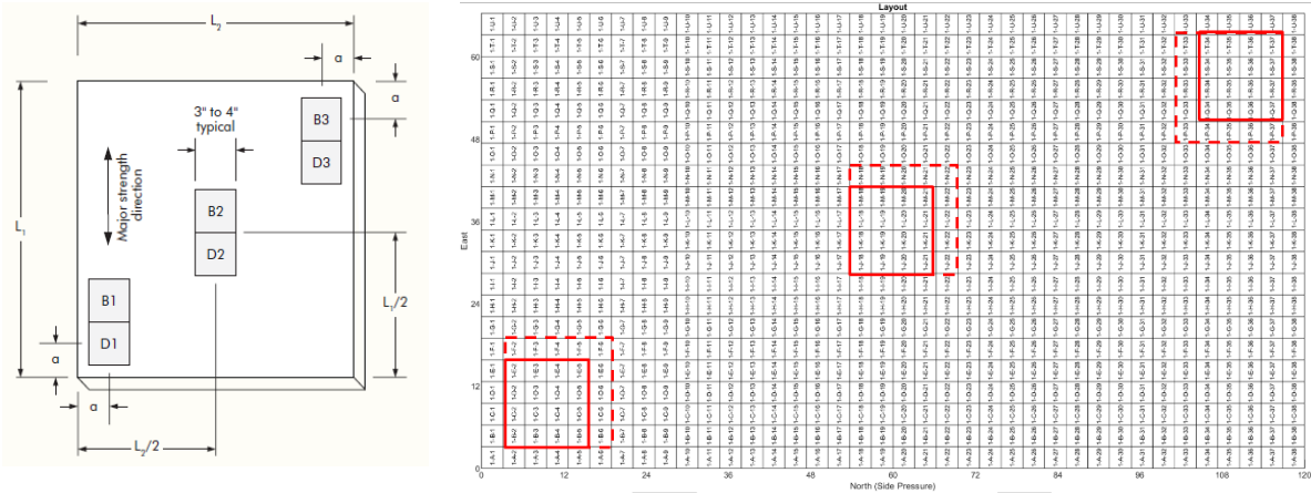
Figure 8. Standard PRG320 sampling scheme for delamination specimens allows more options in small lab-scale billets (left) than in larger test panels (right).
