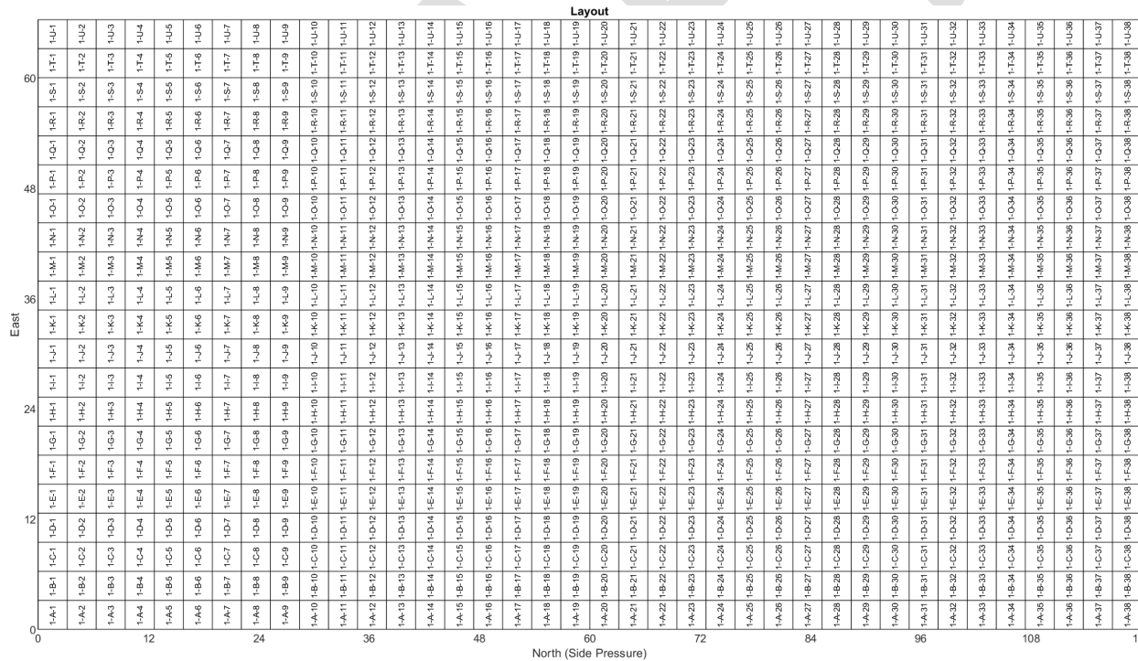
Figure 9. Sub-study panel cutup scheme. In line with original marking, in the subsequent text the horizontal strips are referred to as columns (A, B, C,...) while the vertical strips are referred to as rows (1, 2, 3, ...).
