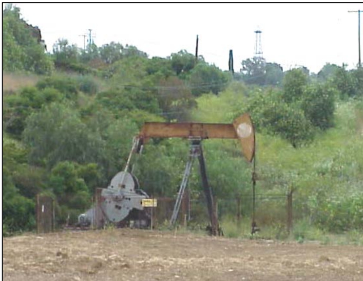
Sucker rod pumping unit extracting oil from a well in Tonner Canyon. Driven by a motor which turns a flywheel with a crank arm, the sucker rod pump can easily lift oil 10,000 feet or more.
