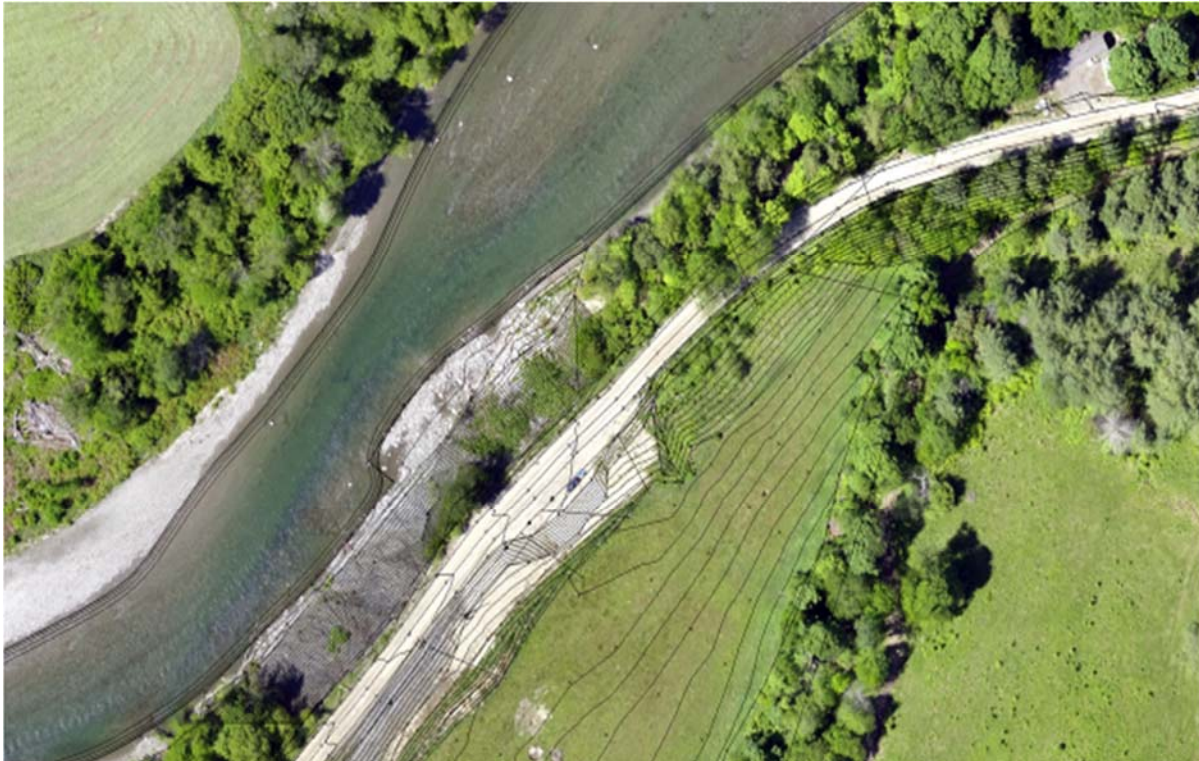
Figure 8. Same riverside area as figure 7 with topography over UAV acquired image-note increased resolution.
