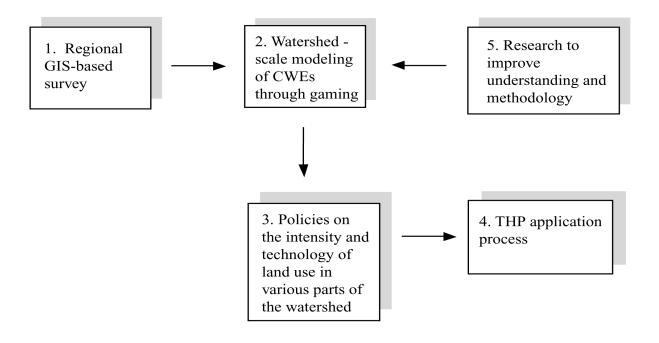
**Figure 1:** The process-based modeling and gaming strategy (Box 2) described in this report would be conducted simultaneously with other decision-support activities, as outlined in the text. Each activity, except for the policy setting (Box 3), would involve a significant component of fieldwork.
