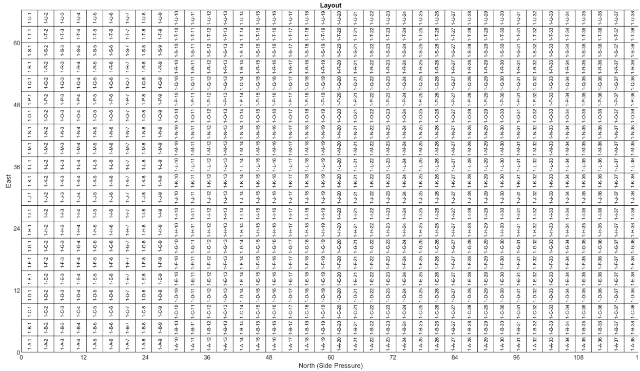
Appendix Figure 9. Sub-study panel cutup scheme. In line with original marking in the subsequent text, the horizontal strips are referred to as columns (A, B, C,...) while the vertical strips are referred to as rows (1, 2, 3, ...).
