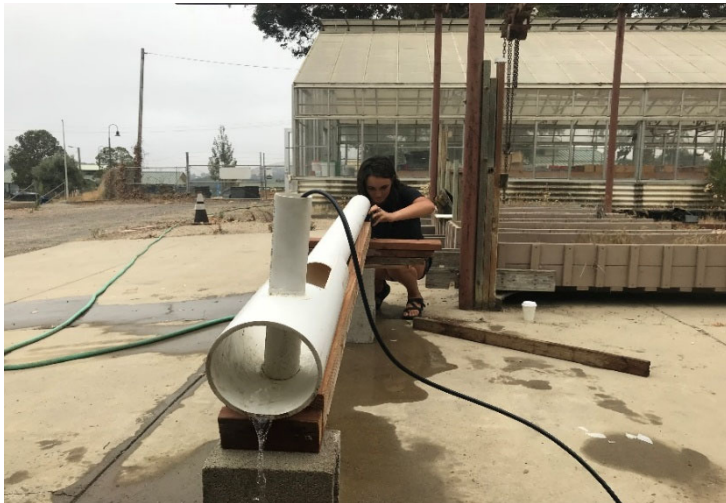
Figure 4. Cal Poly student Grace Goldrich-Middaugh running water into the circular flume to test the stage to water flow relationship. The PVC riser in the center creates a hydraulic jump to allow measurement of stage for flow correlations. The riser also acts as the stilling well for the flume. The cable exiting the riser is the interface cable for a pressure transducer making stage measurements.
