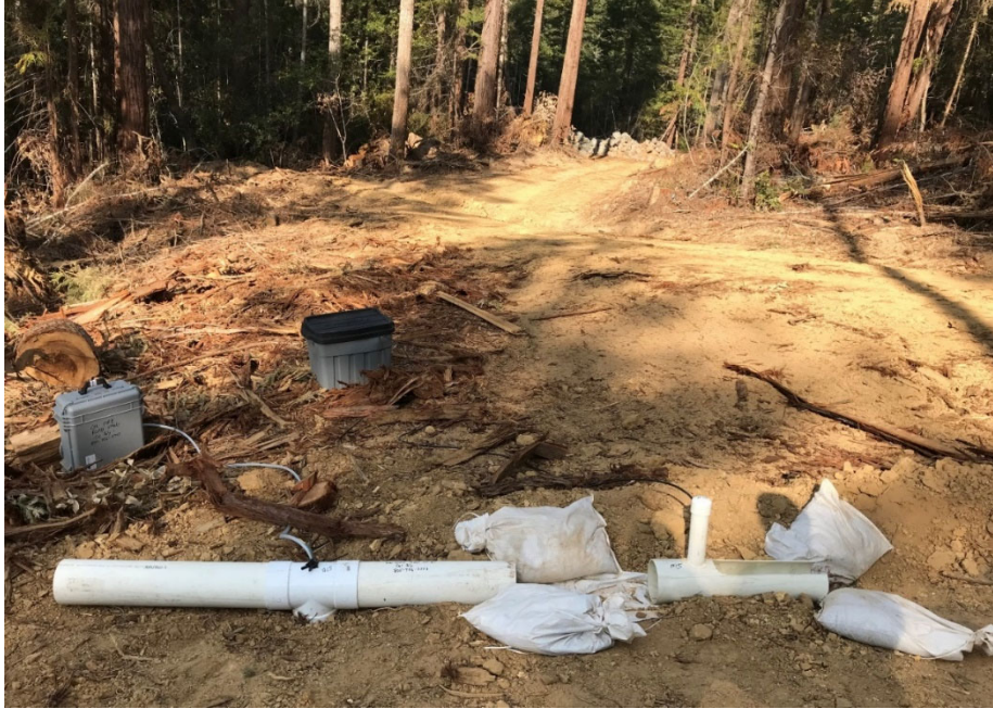
Figure 9. Road site 15 with the initial suspended sediment and turbidity measurement design. The PVC pipe to the left had a T-junction with a reservoir below to allow sufficient depth and mixing of water for sampling. On native surface roads, this design failed due to the reservoir filling with sediment. This design worked on rocky roads with low sediment contributions. The pump sampler is the grey box to the left; the data logger is in the plastic tote.
