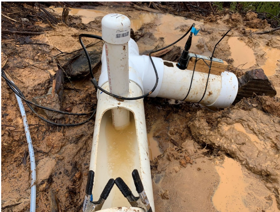
Figure 10. Alternative turbidity and suspended sediment measurement design for high sediment production roads. The reservoir below the road flume is on an angle to pond water and sediment. A drain hole at the end of the reservoir is set at a level that allowed water to pond above the sediment deposition in the reservoir to a depth sufficient for turbidity measurement of the water.
